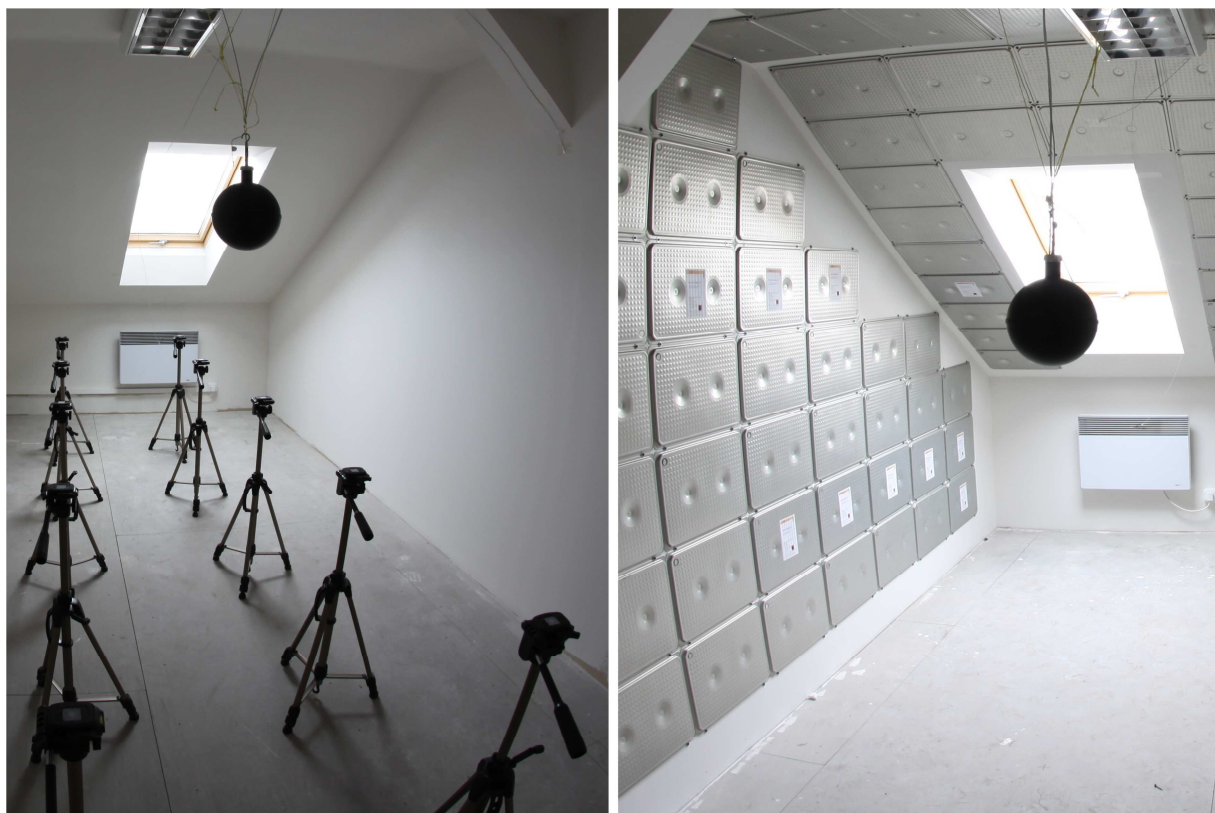
Fig. 28 Figures showing the laboratories [pictures by Ing. D. Bečkovský, Ph.D.] “Laboratory No.1” after the initial positioning of the tripods is on the left, “Laboratory No.2” after the installation of the PCM based panels is on the right.
