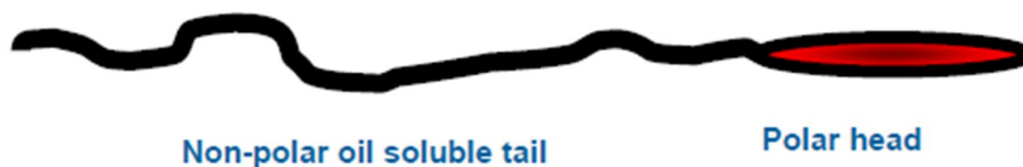
Fig. 6 Schematic representation of a polar additive molecule
