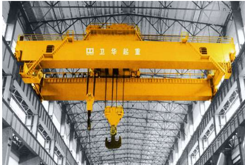
Fig. 9 Heavy overhead crane [36].
