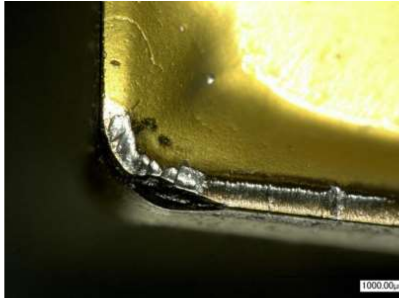
Fig. 65 Tangential insert – Wear after tests.
