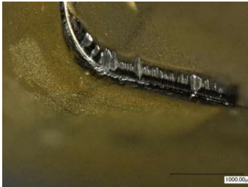
Fig. 64 Triangular insert – Wear after tests.
