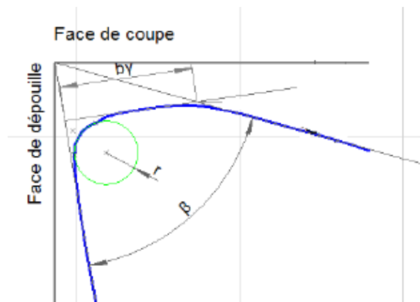
Fig. 49 Side cutting edge geometry of triangular insert.
