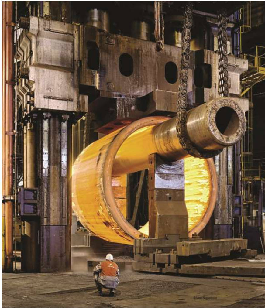
Fig. 41 Reactor pressure vessel being forged in Framatome Le Creusot [49].
