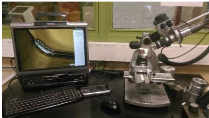
Fig. 58 Tool wear measurement on Keyence microscope.
