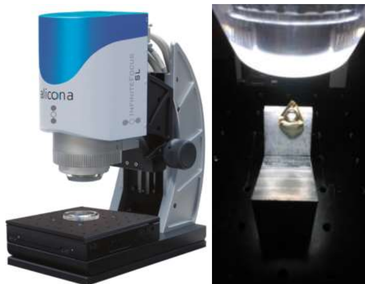
Fig. 43 Alicona measuring device and triangular cutting insert being measured [50].
