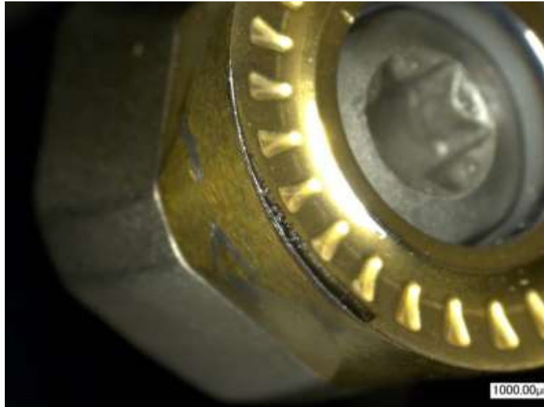
Fig. 63 Round insert – Wear after tests.
