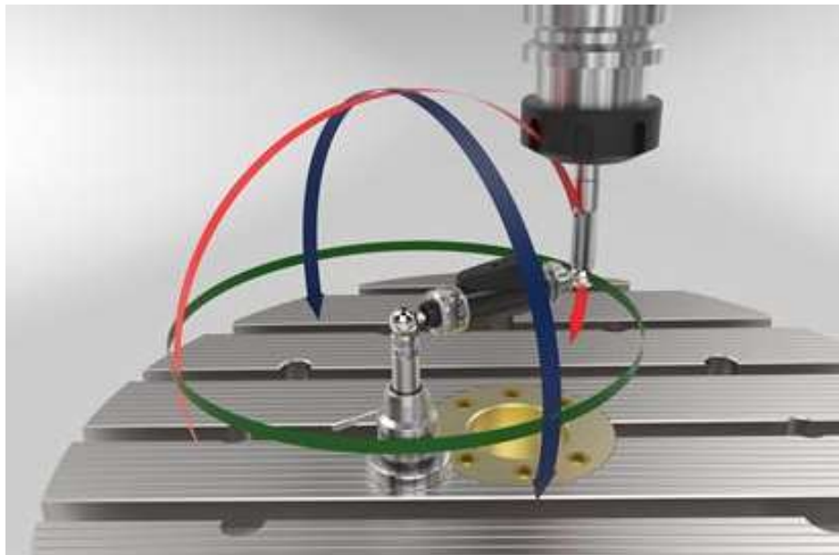
Fig. 40 Ballbar test demonstration [24].
