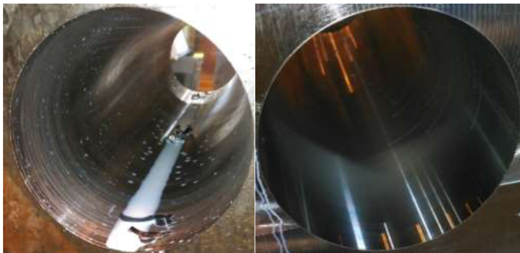
Fig. 13 Comparison of deep drilled hole and finished hole by boring operation.
