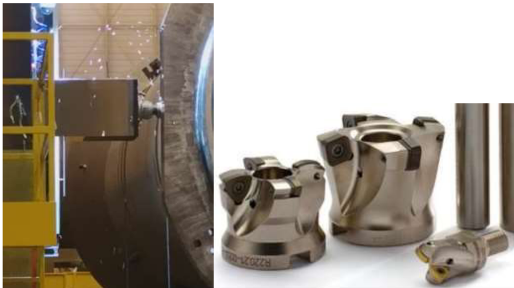
Fig. 17 High feed milling and an illustration of typical high feed milling tools [14].
