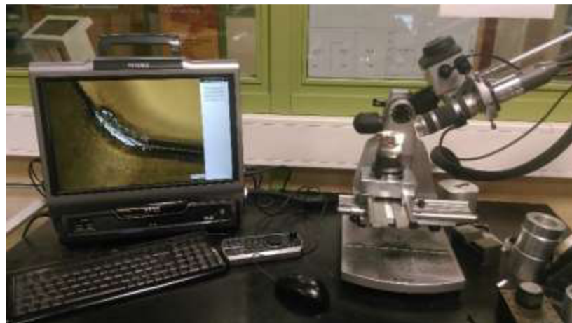
Fig. 58 Tool wear measurement on Keyence microscope.
