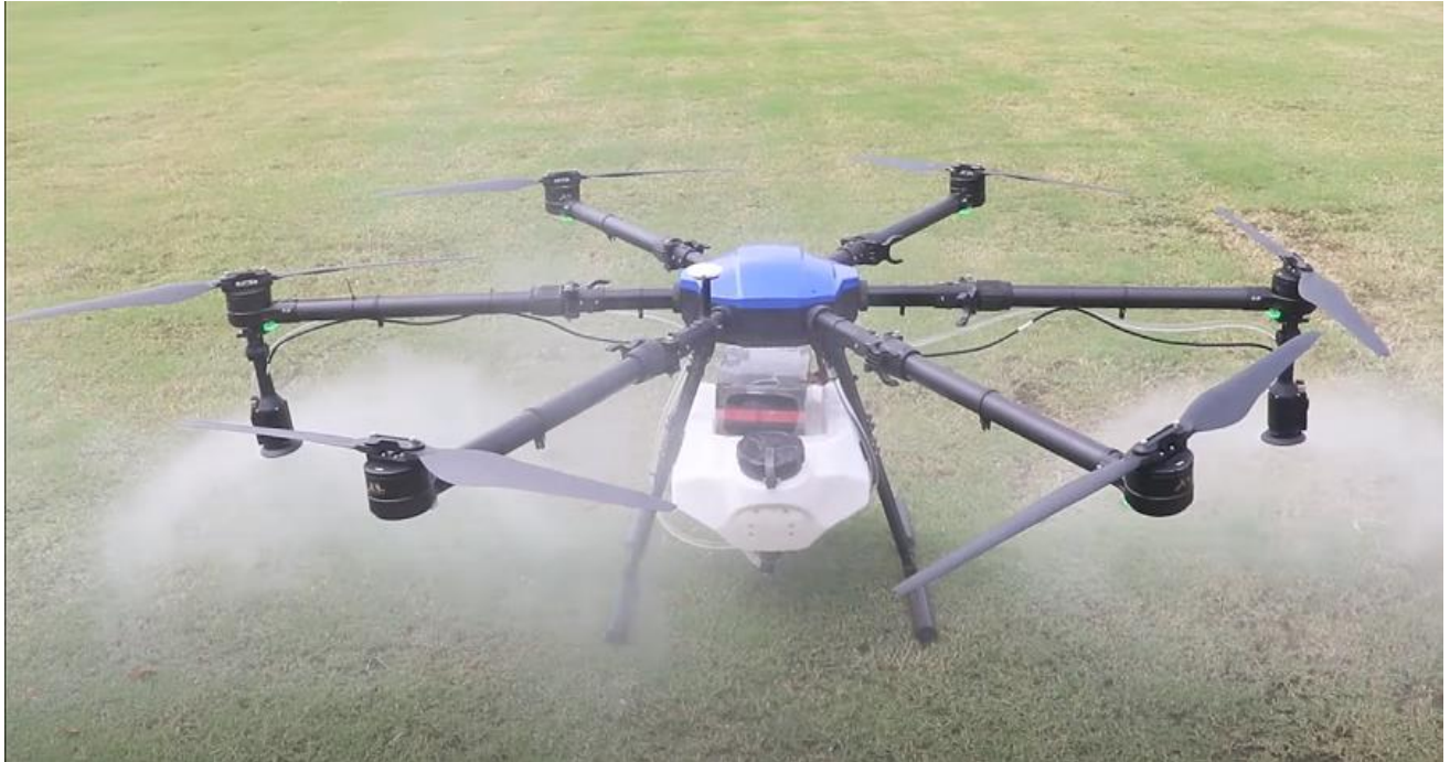
Figure 10. UASS with two centrifugal nozzles.
