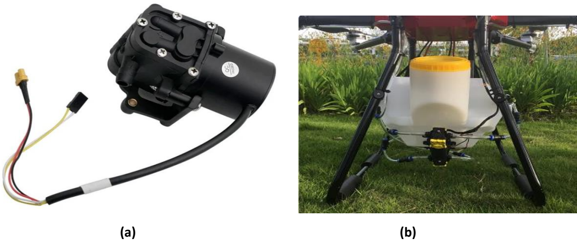
Figure 11. (a) A 3.8 l.min -1 , 24v brushless UAV liquid spraying pump. (b) Mounted pump on a UASS.
