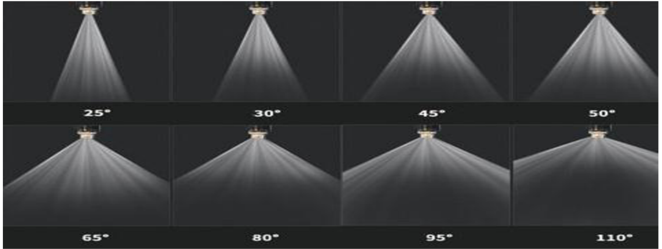
Figure 8. Different angles of convectional nozzle's discharge that define pattern, droplets characteristics.
