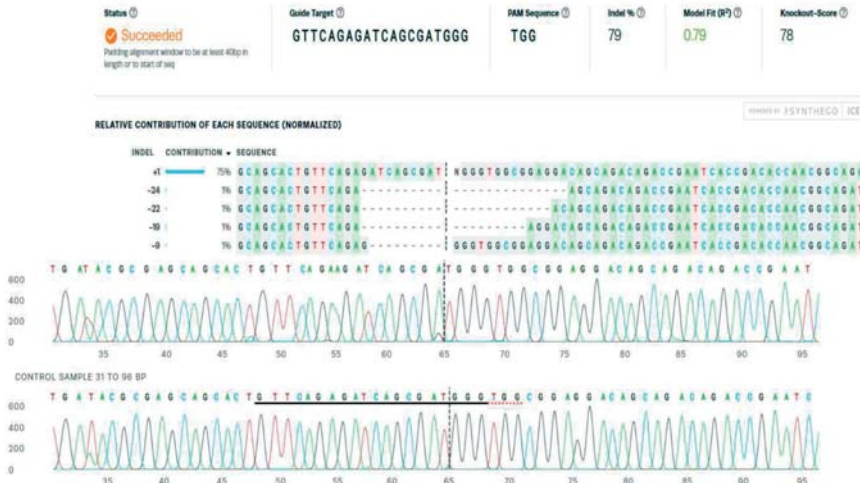
Figure 3. The Inference of CRISPR Edits (ICE) software output of the analyses of the Sanger sequencing data on the fads2 gene part flanking the mutated ATG start codon in fish representative (here, crispant female No. 1) ( ice.synthego.com , accessed on 1 April 2022).
