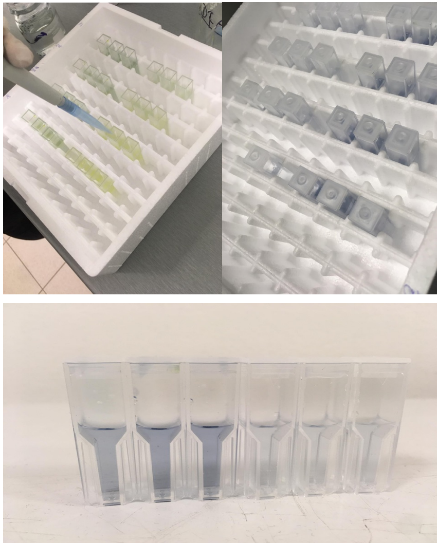
Figure 12. Polyphenol content reaction, changing the color from yellow to blue due phenolic groups contained in the samples (Author)
