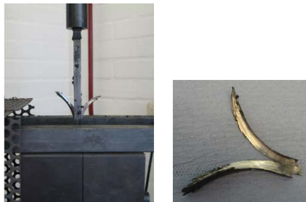
Fig. 5.2 Flow of AZ31 around the plunger.
