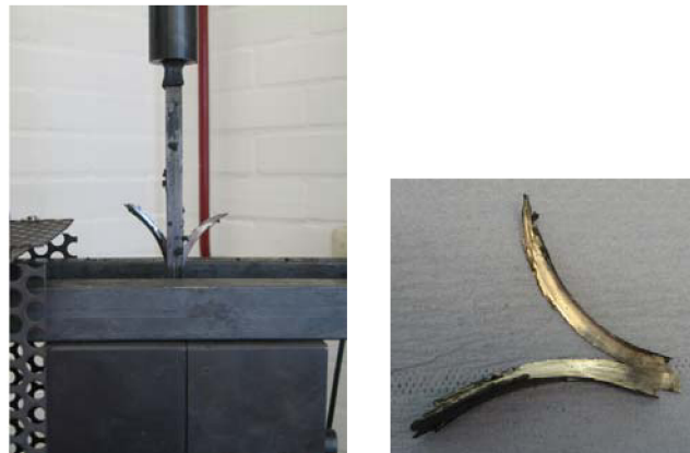
Fig. 5.2 Flow of AZ31 around the plunger.
