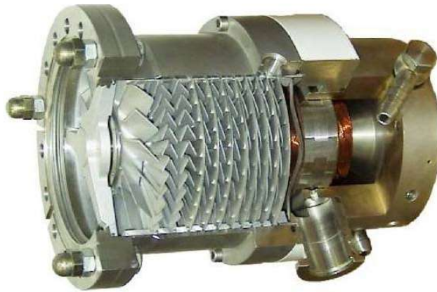
Fig. 1.13: Cross section of a turbomolecular pump driven by a high-speed motor [44].
