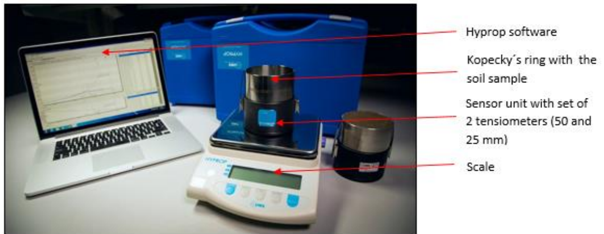
Figure 17. Hyprop device description (adjusted from UMS, 2015).
