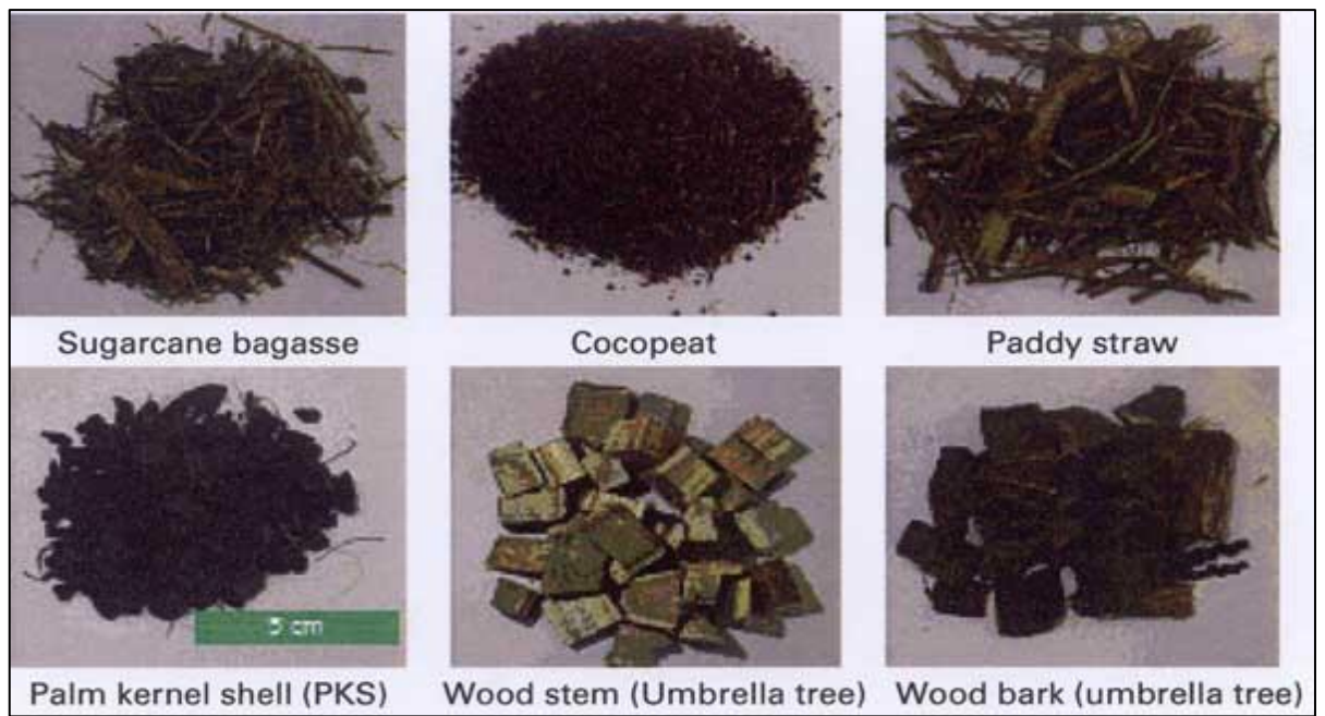
Figure 1. Examples of different types of biomass used for biochar production (Lee et al., 2015).
