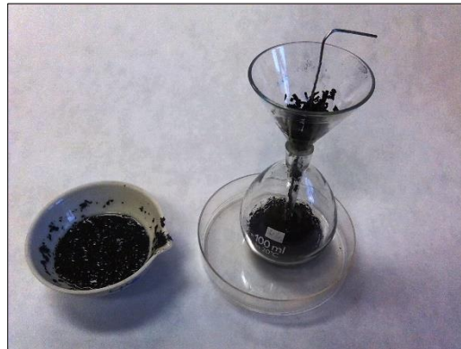
Figure 12. Pycnometer method for determination of particle density of biochar.
