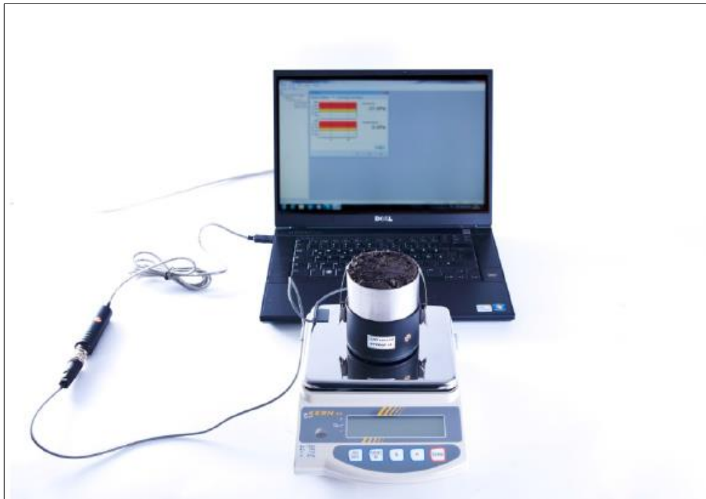
Figure 7. Hyprop device connected to computer with installed SW Hyprop view (UMS, 2015).
