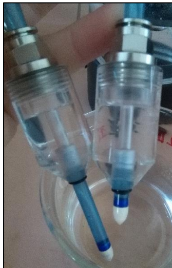
Figure 13. Tensiometer shafts attached to refiling plexiglass components, which were manufactured especially for this experiment.
