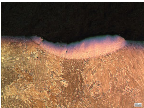
Fig. 37. Sample 10.2. Diameter = 2 mm, speed = 1000 mm/min, gas flow = 40 l/min, power = 1 kW
