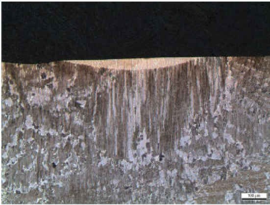
Fig. 41. Sample 12.1. Diameter = 2 mm, speed = 2000 mm/min, gas flow = 40 l/min, power = 1 kW
