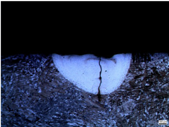
Fig. 28. Sample 8.1. Diameter = 1 mm, speed = 1000 mm/min, gas = 40 l/min, power = 1 kW
