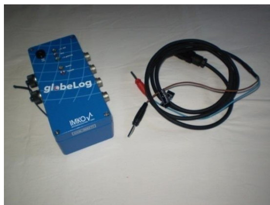
Obr. 3.6 - Datalogger GlobeLog (IMKO GmbH)
