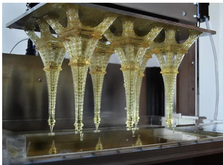
Figure 3 Digital Light Processing [8]
