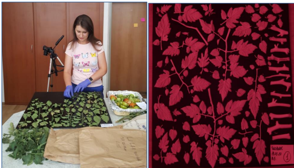
Figure 14. Photographing leaves and stems with a camera with a UV filter
