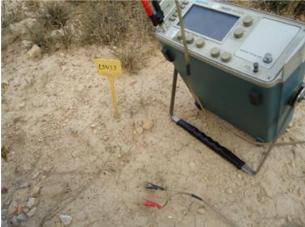
Figure 9. TDR 100 connected with sensors to metal rods. Reprinted with the permission of the author (Lalaguna, 2016)
