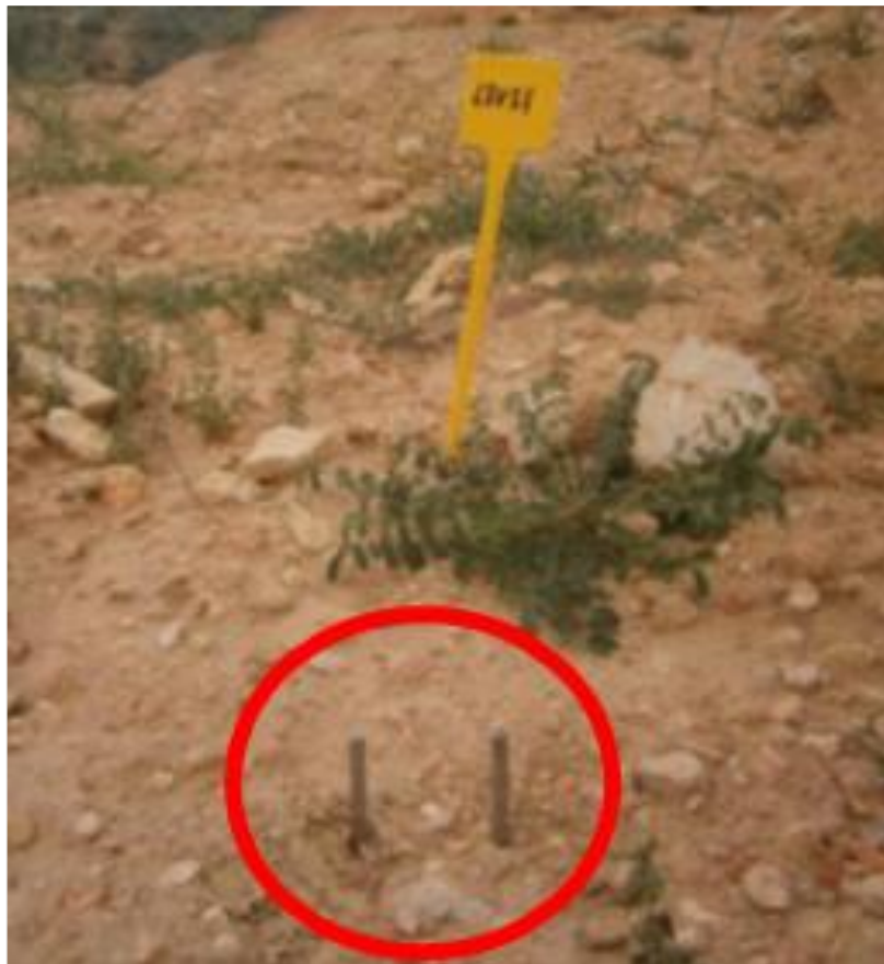
Figure 8. Pair of metal rods 20 cm deep into the soil. Reprinted with the permission of the author (Lalaguna, 2016)
