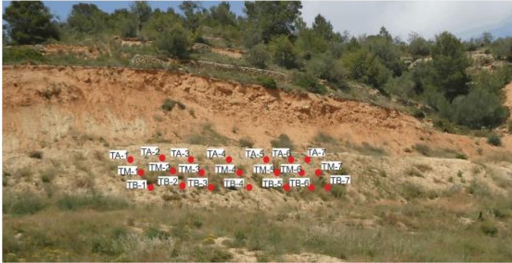
Figure 11. Distribution of sampling points in the slope restored by the conventional approach in Aurora quarry. TA: top of the slope, TM: middle slope, TB: Bottom slope. Each transect had seven sampling points. Reprinted with the permission of the author (Lalaguna, 2016)
