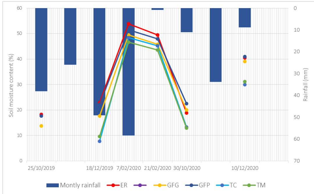
Figure 21. Monthly rainfall amount and SMC in each treatment during the recharge period in the Fortuna Quarry. ER: Reference ecosystem area, GFG, GFP: two units of geomorphic restoration treatment, TC, TM: two different units of conventional restoration treatment
