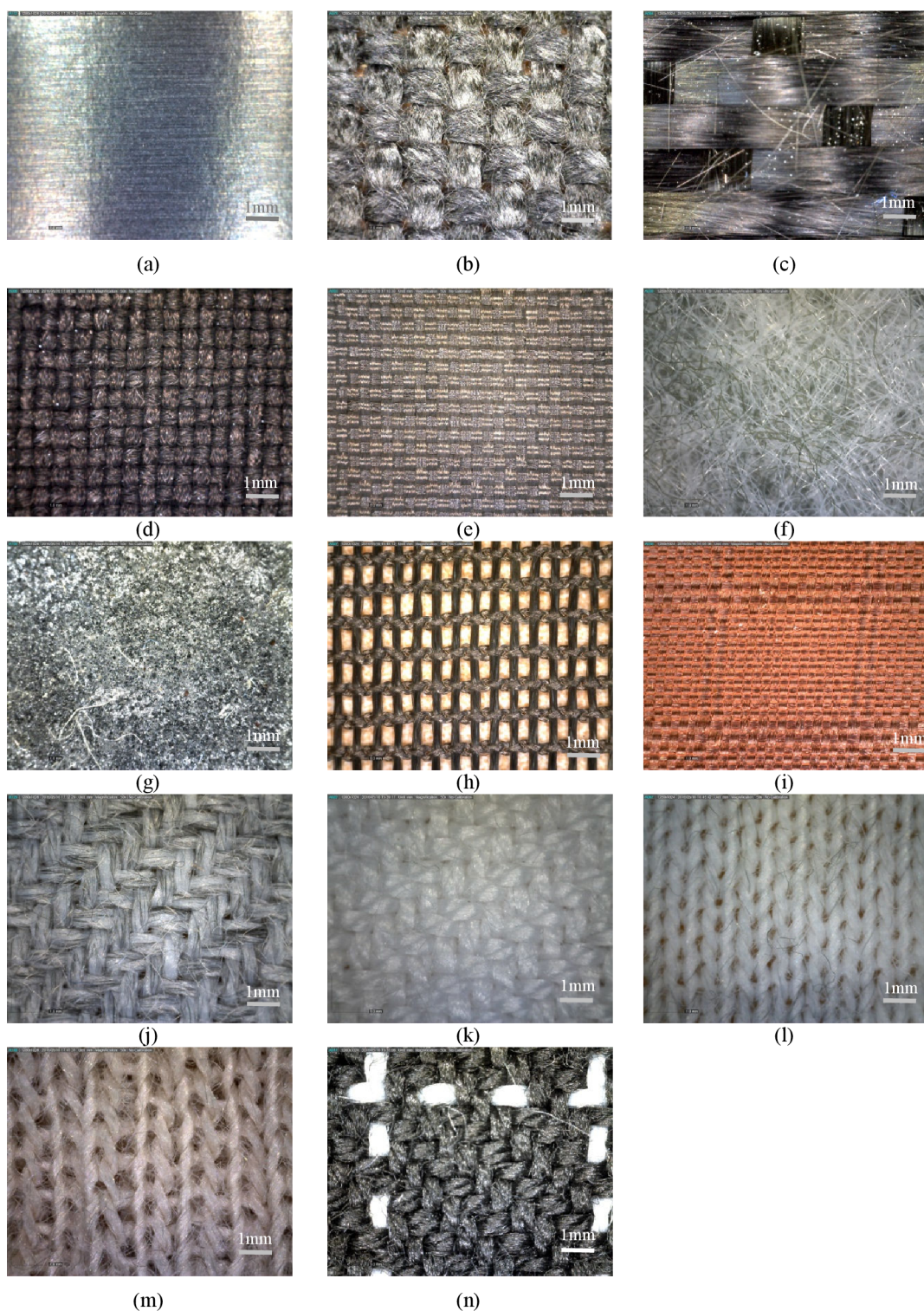
Figure 15. Microscopic images at 50x magnification of electrically conductive sample set. (a) Aluminum foil, (b) “Ca W 1”, (c) “Ca W 2”, (d) “PPy/PES W”, (e) “Mf Ag W”, (f) “Mf 20Eu NW”, (g) “Mc Al NW”, (h) “Mc Ag K”, (i) “Mc Cu/Ag W”, (j) “H 20SS W”, (k) “H 1SS W”, (l) “H 15SS Ks/j”, (m) “H 10SS Kd/j”, (n) “H 10SS WG” [1].
