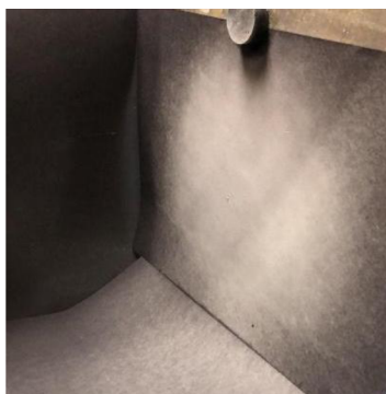
Figure 44 Observation of fibre formation on a paper attached to the collector.
