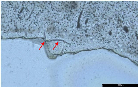
Fig. 7.18: Sample B. Microcrack penetrating under the surface irregularity indicated by red arrows. Magnification 100×, scale bar 300 μm (photo SB).
