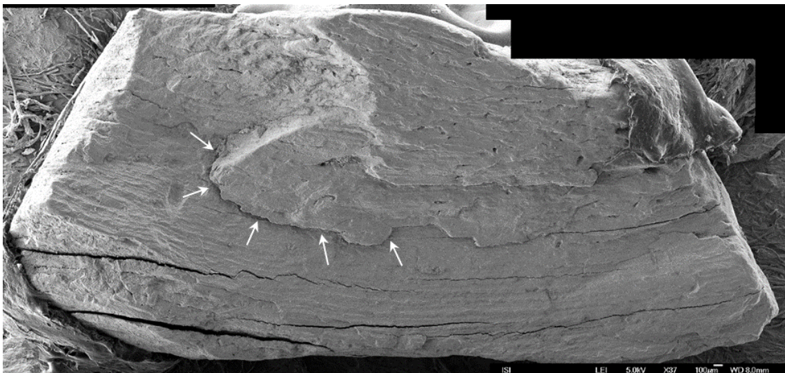
Fig. 8.27: Sample A8. Plate-like protrusion lined by cracking (white arrows). Magnification 37 \times , scale bar 100 \mu m (photo Z. Pokorná and SB).
