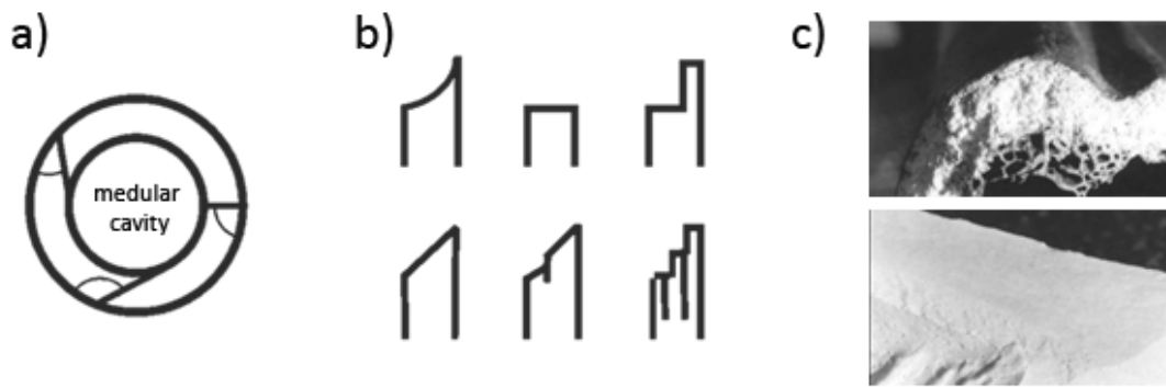
Fig. 6.1: Illustration of evaluated traits, a) angle of the fracture surface in relation to the outer/inner bone surface, b) outline of fracture, c) rough (upper) or smooth (lower) character of the fracture surface ( Outram 2002, 54-55, Fig. 6.2, 6.3 6.4, 6.5, modified by SB ).
