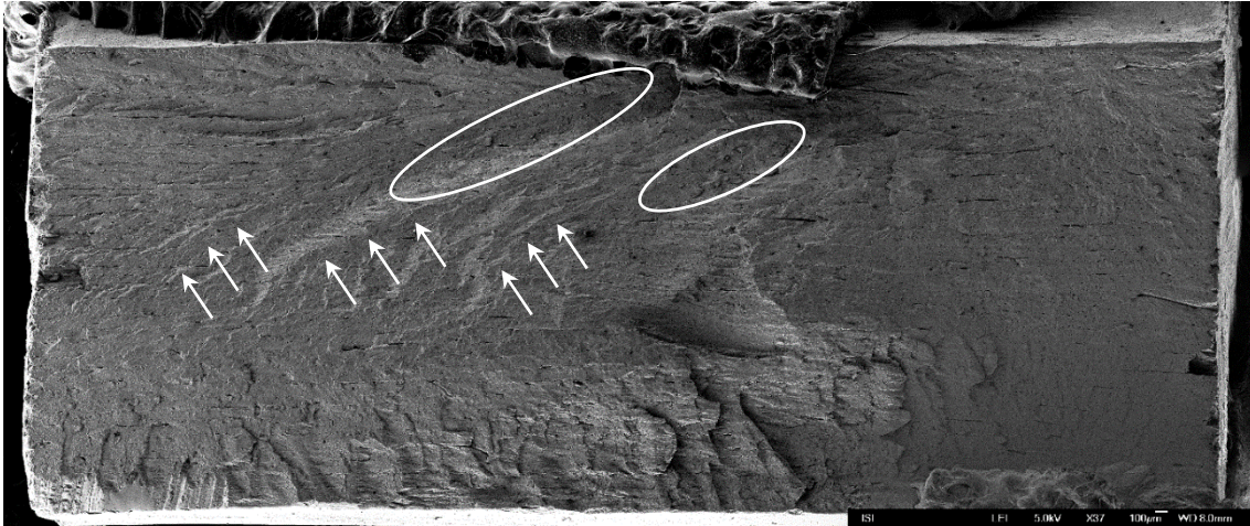
Fig. 7.53: Sample IOTA. Granular areas (white circles) near to clearly visible arcuate ridges forming the fan-shaped pattern (white arrows). Magnification 37 \times , scale bar 100 \mu\text{m} (photo Z. Pokorná and SB).
