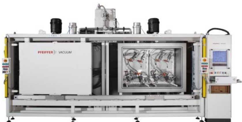
Obr. 11) Pfeiffer Vacuum testovacia jednotka chladiacich hadíc [11]
