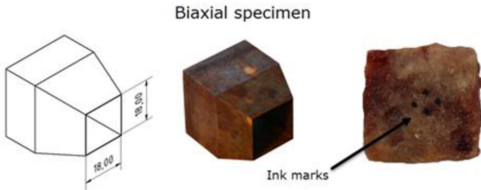
*Figure 24 Dimensions [mm] of tested biaxial specimen*
