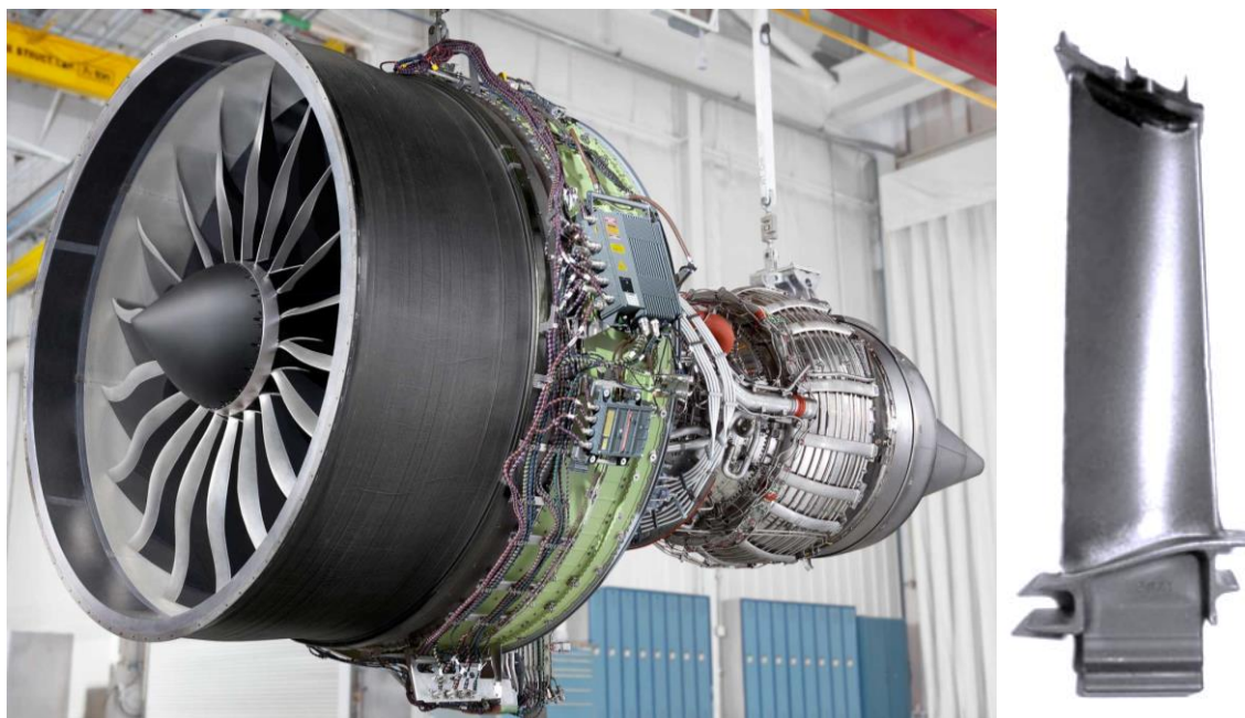
Obr. 8 Turbína Genx-1B a TiAl lopatka [13],[14]
