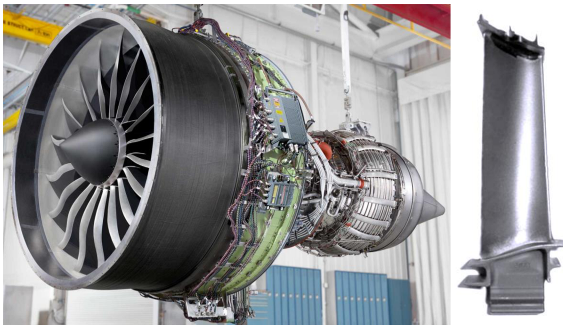
Obr. 8 Turbína Genx-1B a TiAl lopatka [13],[14]
