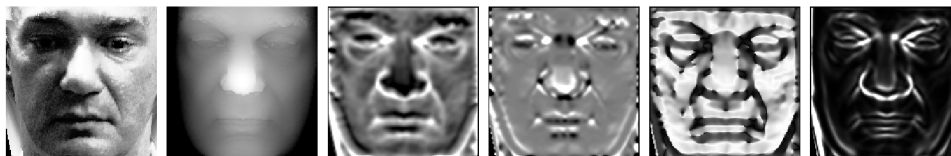
Figure 5.4: Image representations of the face surface. From left to right: texture, range image, mean curvature, Gaussian curvature, shape index image, eigencurvature.
