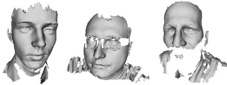
Figure 3.3: The examples of scans obtained with the Artec 3D M scanner. The structured light scanners have a problem with scanning shiny objects or a structure where the projected pattern is highly distorted. This problem leads to the impossibility of capturing glasses (middle scan) or a beard (right scan).
