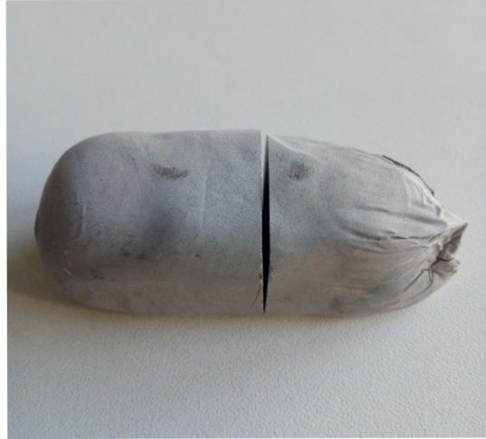
Figure 4.7: The sample after the CIP underwent 500 MPa for 5 minutes.
