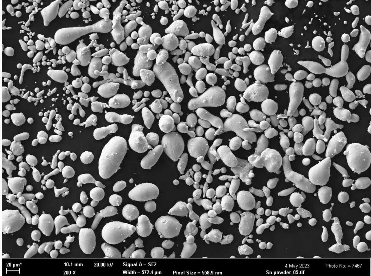
Figure 4.6: SEM image of Tin powder, magnification 200x, SE detector.
