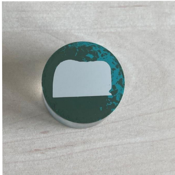
Figure 4.8: The sample after the grinding and polishing
