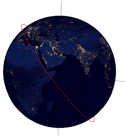
Figure 5.1: Here is the Earth spherical model (excluding Equator oblateness) with ECI coordinate axis X, Y, Z colored red, green and blue, respectively. Red ellipses capture 10 unperturbed Keplerian orbits computed from raw space-track.org data. Transparency indicates evolution in time, where opacity increases proportionally with time.
