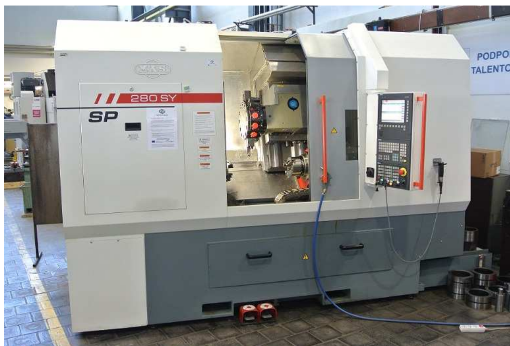
Obr. 5.4 CNC soustruh MAS SP 280 SY.
