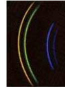
Fig. 7 Emissive bars of mercury lamp
