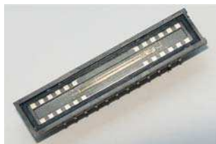
Fig. 2 Linear line image CMOS sensor Hamamatsu S10077.
