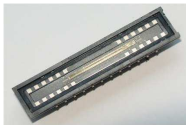
Fig. 2 Linear line image CMOS sensor Hamamatsu S10077
