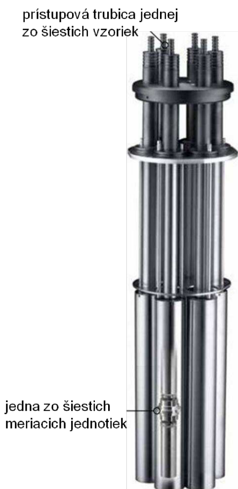
Obr. 7: Meriaca cely multikalorimetra so šiestimi minikalorimetrami [65]
