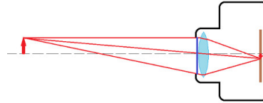
Figure 2.5: Lens in camera focus light from one point in scene into one point in sensor [4]
