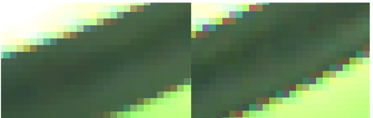
Figure 4.4: Difference between Freeman(left) and Bilinear(right) debayering
