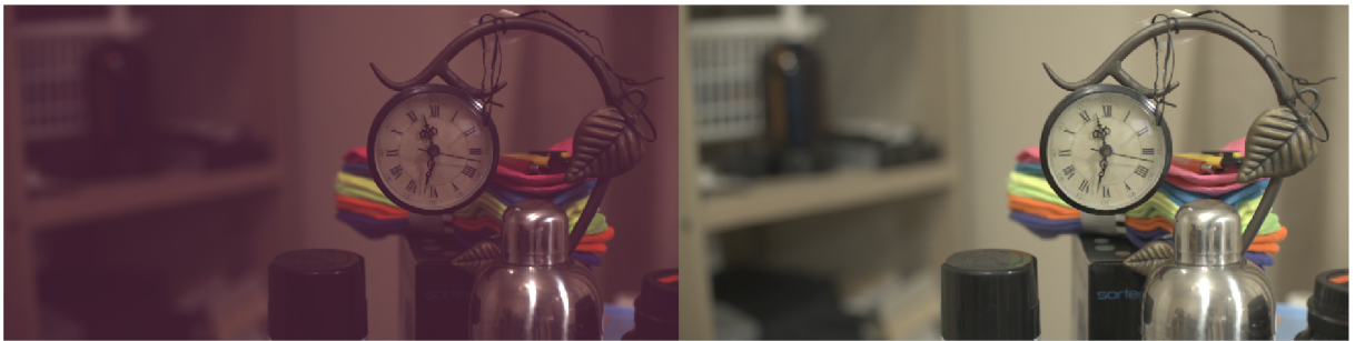
Figure 4.5: Image on the left side is processed without linearization (too much red color) and on the right side is with linearization
