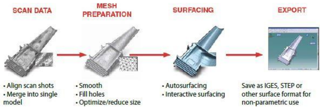
Figure 8. Scan to surface process[19]
