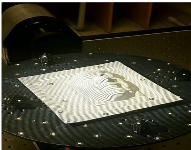
Figure 5. Projection of strips lights
