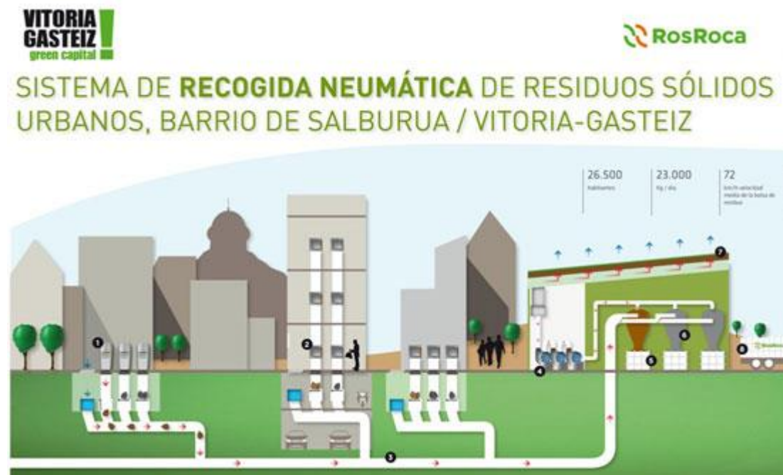
Figure 11. System of pneumatic collection of residual waste in distrikt Salburua (Vitoria-Gasteiz, online)
