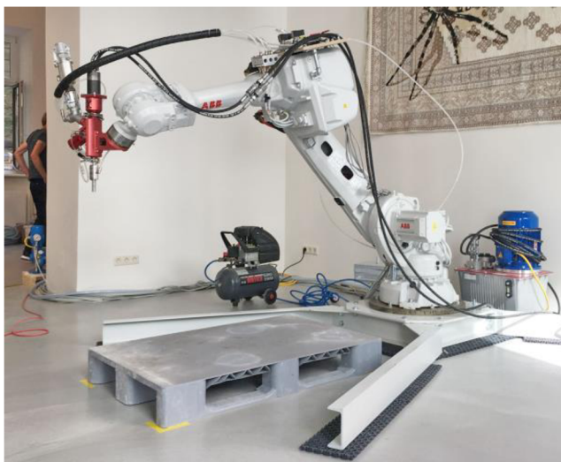
Obr. 2 3D tiskárna BauMinator® [4]
