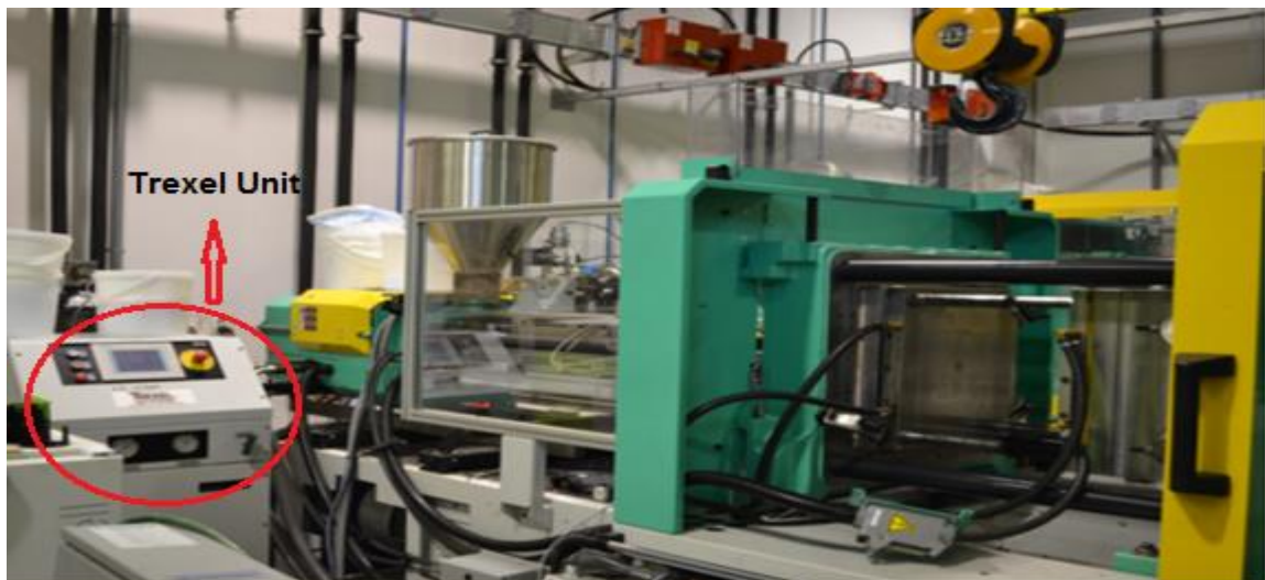
Fig. 11: Injection moulding machine and Trexel unit for foaming process
