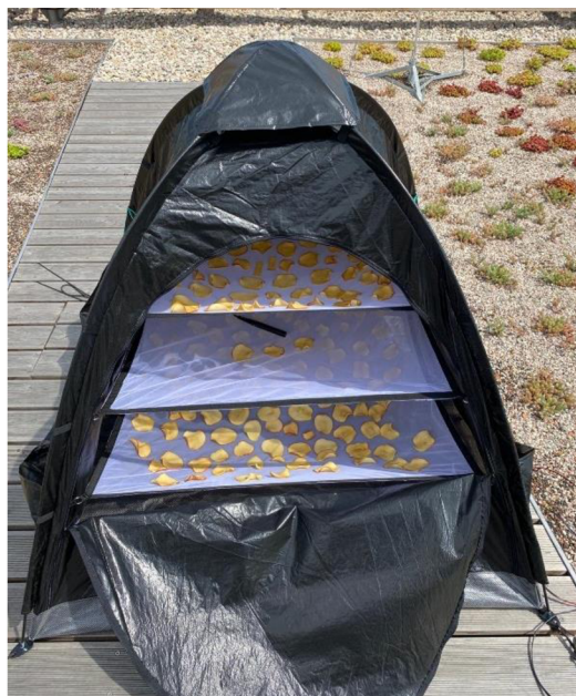
Figure 15: Indirect solar dryer filled with apple samples
