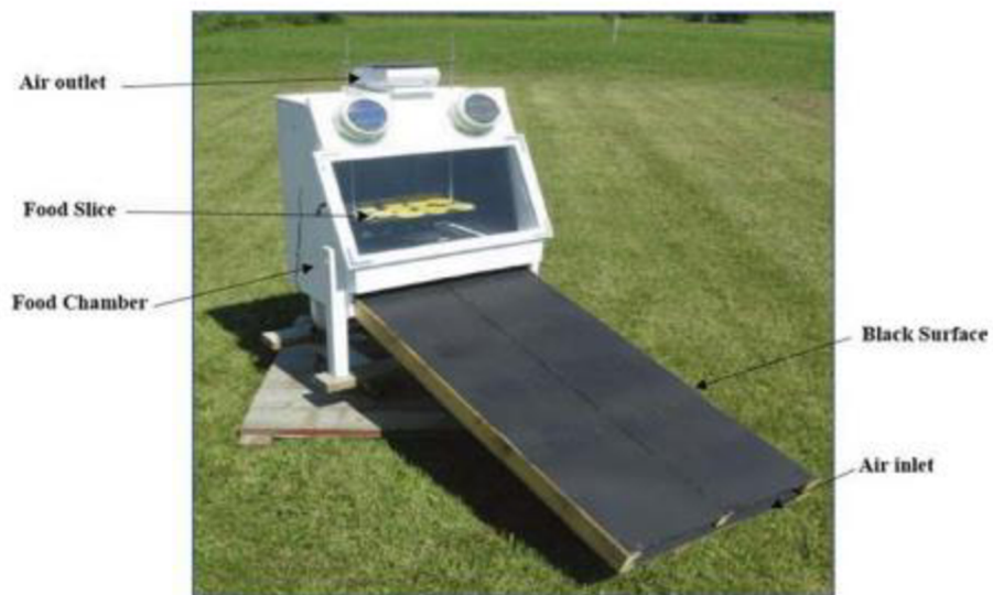
Figure 10: Closed solar drier (Masud et al. 2020)
