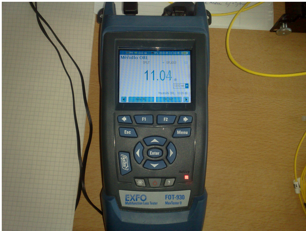
Fig. 34: the test meter FOT-930 measuring ORL in the laboratory.
