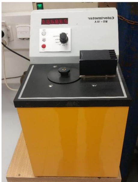
Figure 21. Picture showing MS-10A calorimeter.
