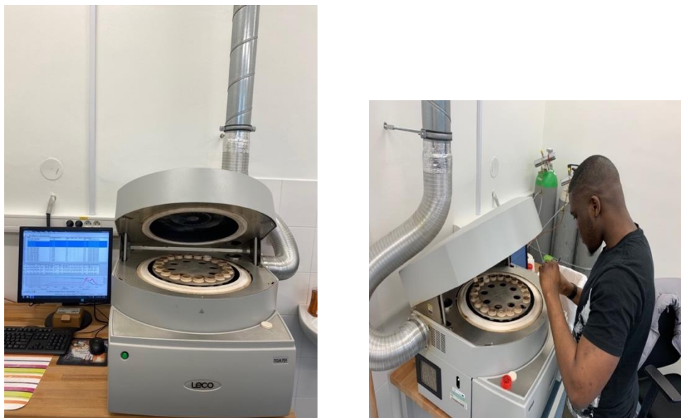
Figure 27. Picture showing weighing furnace LECO TGA 701.
