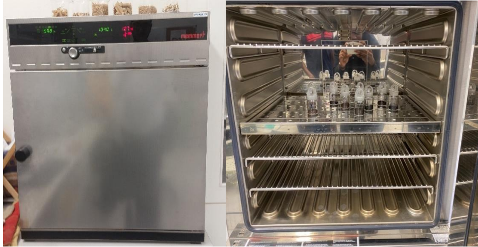
Figure 20. MEMMERT drying oven (Model UFE 500) with coconut husk samples.
