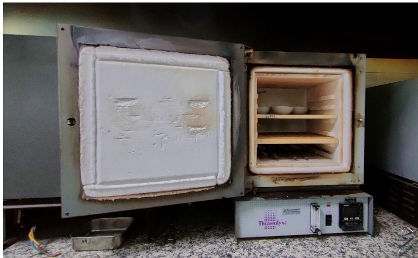
Figure 23. Dry samples tested in muffle furnace.
