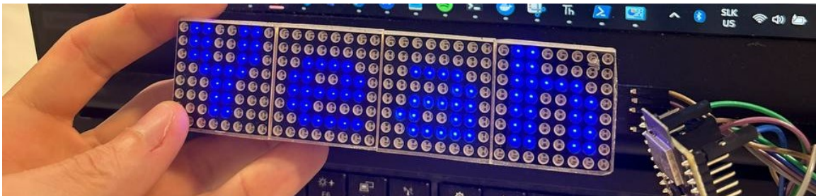
Figure 7.6: Illustration of the LED Matrix showing expected output.
