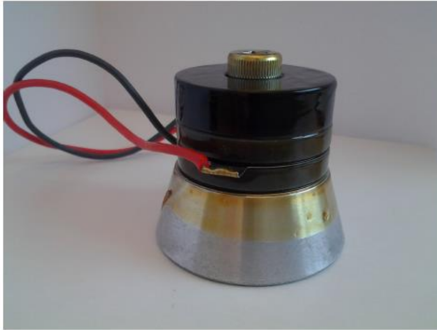
Figure 1.9: Piezoelectric transducer for ultrasonic cleaning
