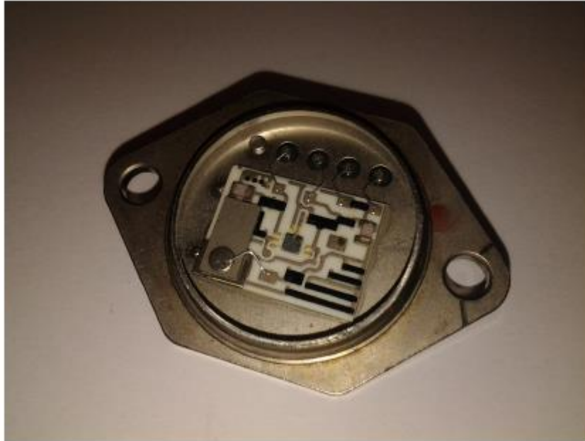
Figure 1.7: Piezoelectric acceleration sensor
