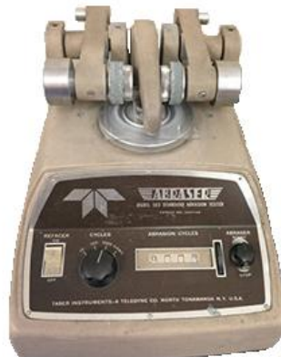
Obr. 10: Taber-Abraser, model 503 Standard ( http://www.taberindustries.com )
