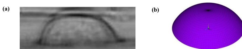
Figure 4. 8: Typical images of: (a) an adherent cell on a rigid microplate [50] and (b) corresponding proposed FE adherent cell model.
