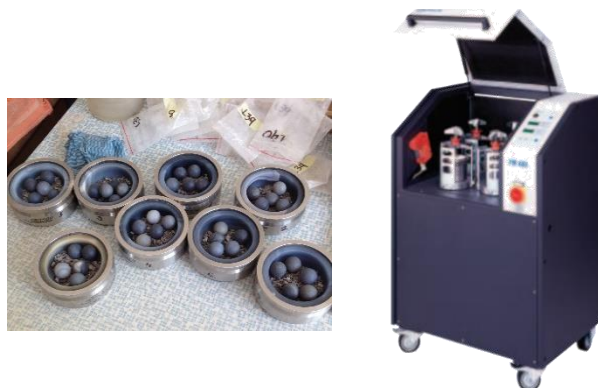
Figure 9. Left: Agate balls. Right: Mill for homogenization of samples.
