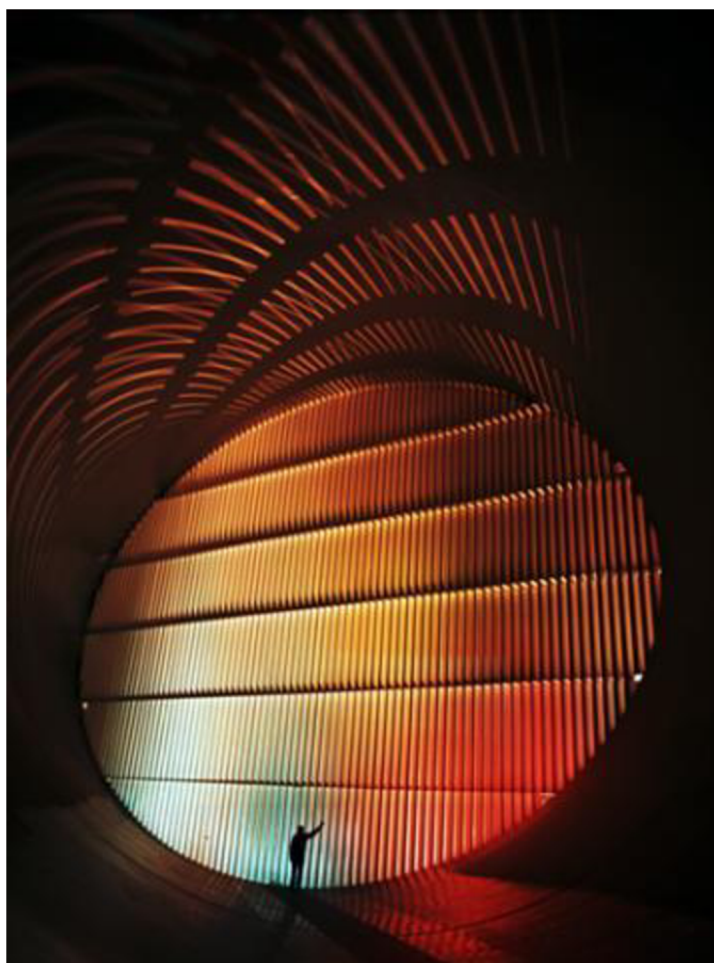
NASA 16 Foot Transonic Tunnel Turning Vanes NASA Langley Research Center 5/1/1990 Image # EL-1996-00006
