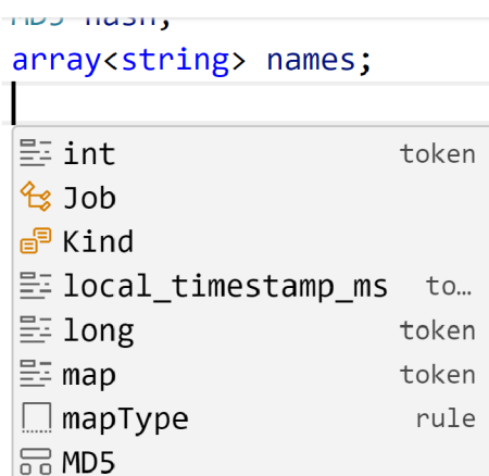
Figure 6.4: Code completion menu after adding a simple CompletionHandler that offers items from the symbol table as suggestions.
