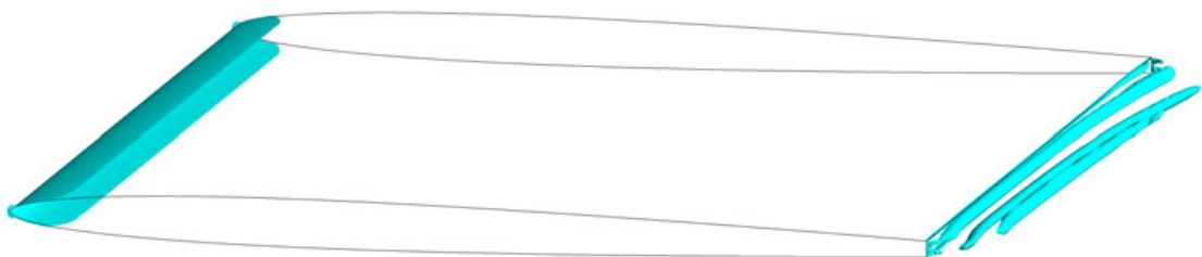
A 1.6 Vortex shedding at v_{inlet} = 5 \text{ ms}^{-1} visualised by iso-surface of Q-criterion for value 2.5 \cdot 10^6 \text{ s}^{-2}
