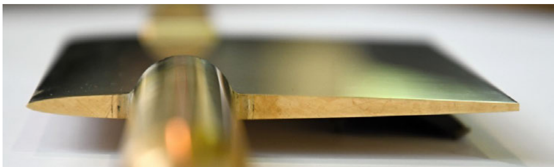
Fig. 6.4 Photo of the hydrofoil made of brass
