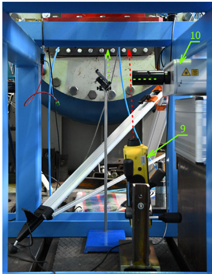
Fig. 6.18 LDV laser beam (red); PIV laser (green) - a mirror creates laser plane
