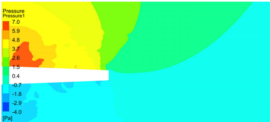
A 7.1 Pressure field from unsteady CFD with prescribed motion at v_{inlet} = 0 \text{ ms}^{-1}
