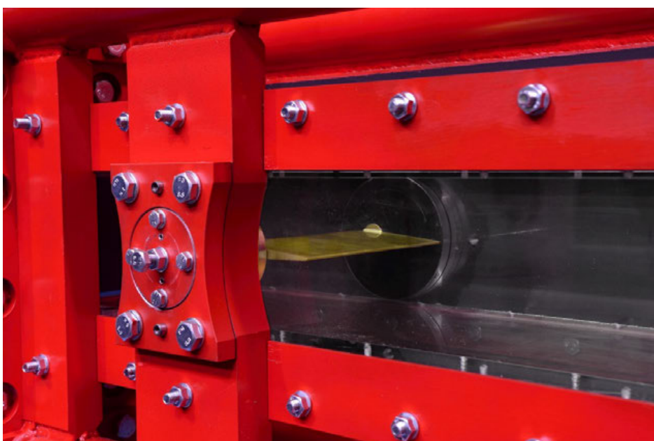
Fig. 1.1 Hydrofoil placed into the cavitation tunnel
