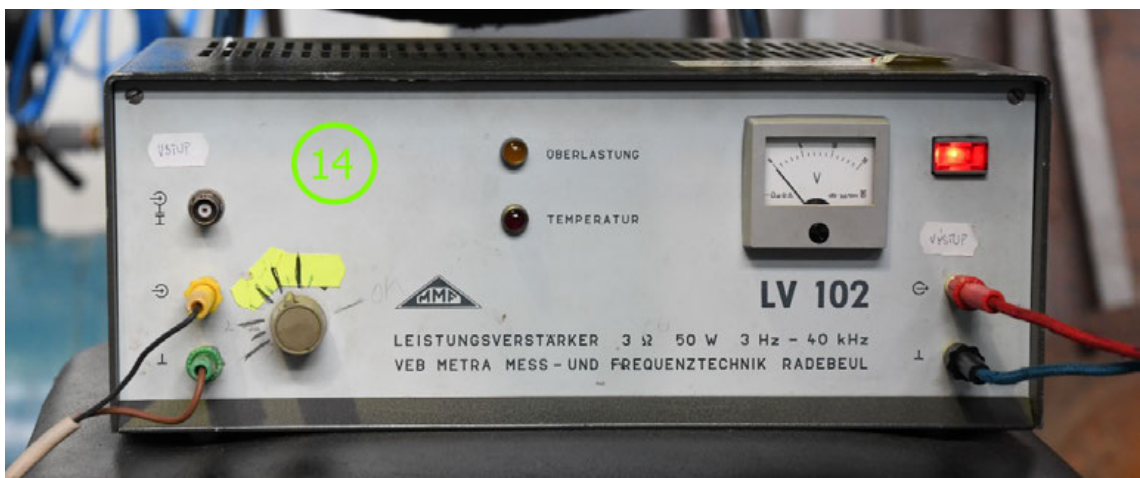
Fig. 6.14 Power Amplifier which amplifies the input signal of external exciter
