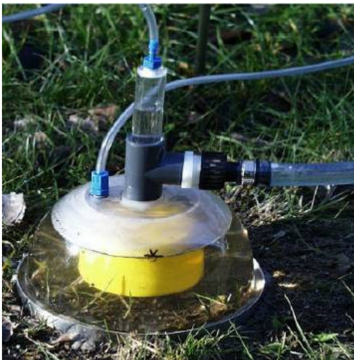
Figure 20 - Excess of sand between the hood and the outer ring of HI, UGT GmbH [online]
