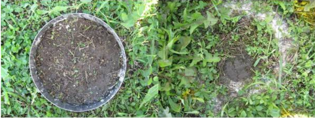
Figure 19 - Prepared place for measurements - trimmed grass on the place for the HI and for MDTI, which was put on the same place as the Hood after about a week when the soil water content had settled to the the previous conditions as much as possible
