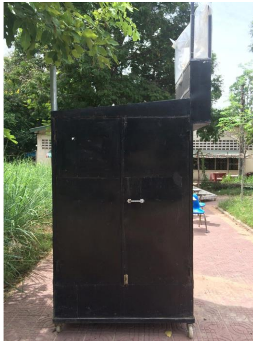
Figure 12.B Picture of hybrid solar dryer (HSD) (Source: Nikola Ždímalová, 2015)
